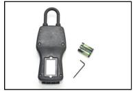
4. Remove the two small screws that hold the battery cover on the back of the lockbox. You will need either a 5/64" hex/allen wrench or a T10 torx driver to remove the screws. You may be able to borrow these tools from your Association.
