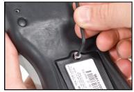
5. Once you remove the screws, the battery cover should come off and reveal the 2CR5 type lithium battery. Observe the orientation of the old battery.
