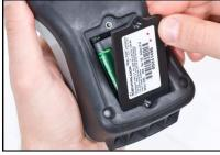
6. To remove the battery, turn the lockbox face up. Tap the keypad side of the lockbox against the palm of your hand. This should dislodge the battery from the back of the lockbox. If the battery does not dislodge, tap the keypad side of the lockbox against a hard surface. Place the lockbox over a table before attempting to remove the battery. Do not let the battery fall to the ground. Be careful not to bend the battery contacts.
